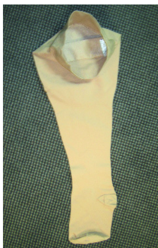
FIGURE 39 Circular knit knee high garment Shaped by varying yarn tension and stitch height during knitting.
