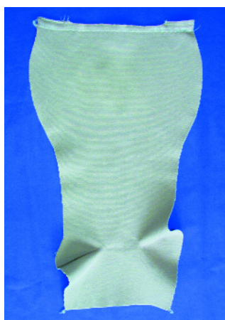
FIGURE 40 Flat knit knee high garment before sewing Shaped by adding and removing needles during knitting.
